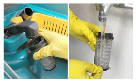
**B.** Remove debris tray from machine. Dispose of debris in waste container and rinse out tray. Reinstall debris tray.
