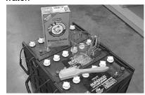
**2.** Check for loose or corroded battery cables.
