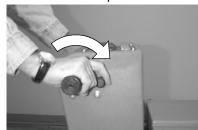
**(2550 model)** Pull reverse trigger to operate machine in reverse.
