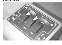
**STEP 5:** To begin burnishing, roll control handles forward. **(2550 model)** Turn speed control knob to desired speed.
