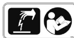
ELECTRICAL COMPONENTS, USE GROUNDING STRAP BEFORE OPENING PANEL LABEL - Located on electrical panel under seat
