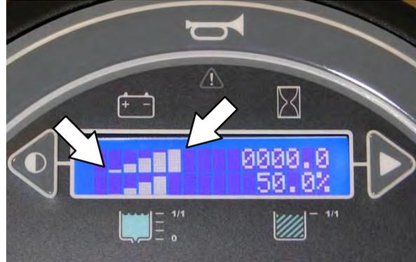
When the batteries are fully charged, all five bars are lit. Recharge the batteries when there is only one bar shown in the display. Do not allow the batteries to discharge below the last bar.
