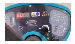
Use the + and – switches for solution flow adjustment to change the CD%.
