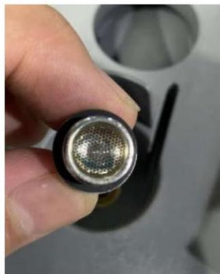
Assemble the washed filter joint on the machine and tighten it with the #2 hex wrench.
